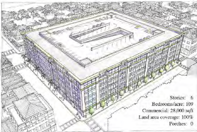
This image illustrates a 6-story “Texas donut” style mixed-use building wrapped around a parking garage. It is built to the property line and maximizes the allowable footprint.
