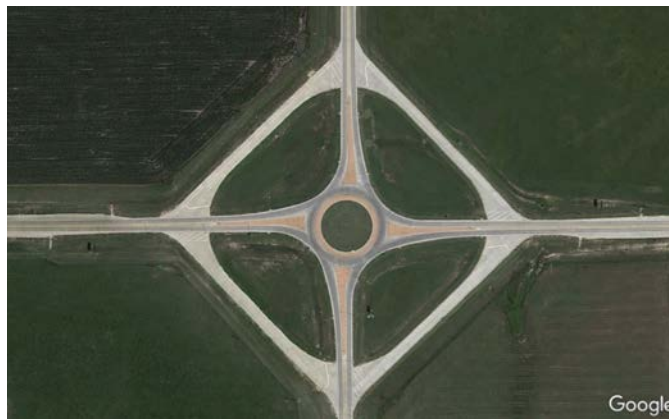
Exhibit 10.40. Example of OSOW bypass lanes.
