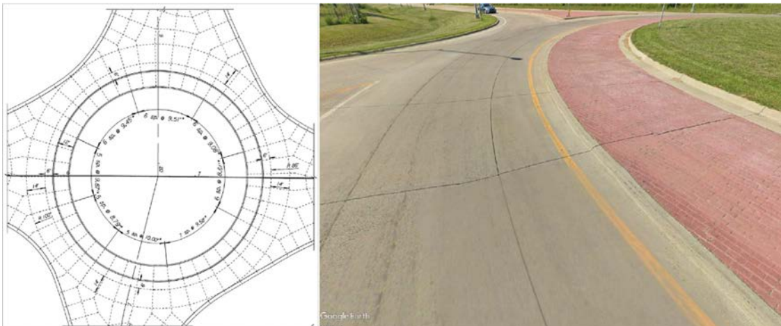
Exhibit 13.6. Example jointing plan for a single-lane roundabout.
