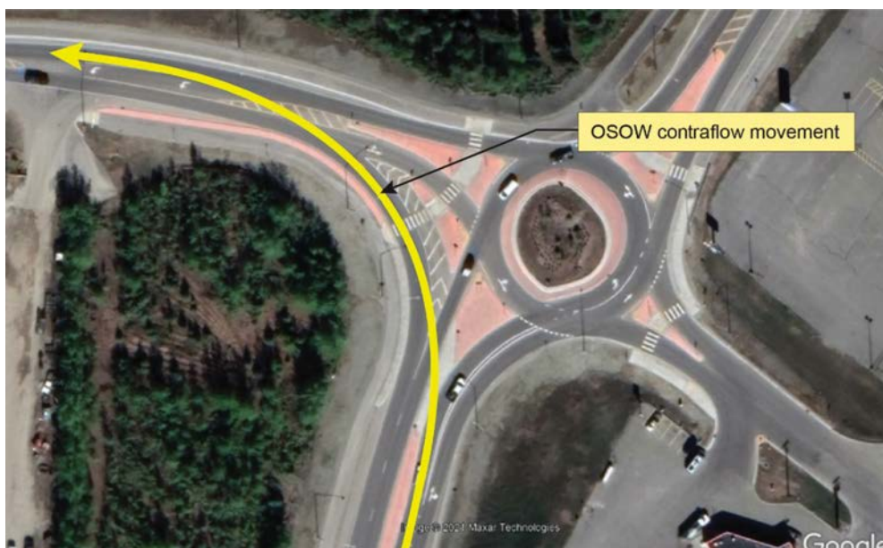
Exhibit 10.41. Example of OSOW contraflow movement using a bypass lane.
