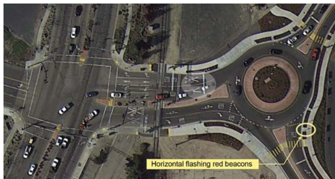
Exhibit 12.34. Example of aerial perspective of railroad crossing near roundabout.
